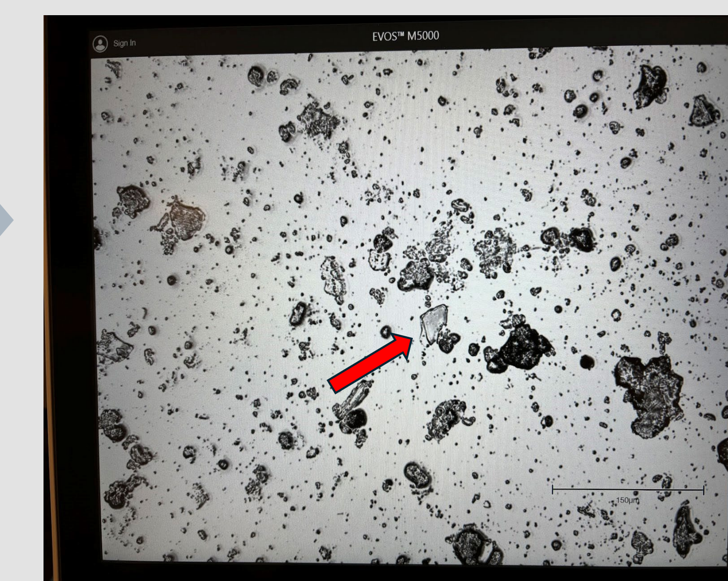
Unstained fluorescent microscopy of 7-month mature compost with TRANS UV - an arrow indicates a film microplastic
