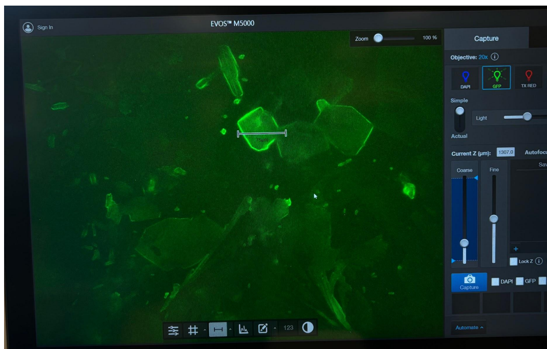
Figure 4. Stained microplastic fragments under x20 magnification of the fluorescent microscope, digested with 10% KOH..
