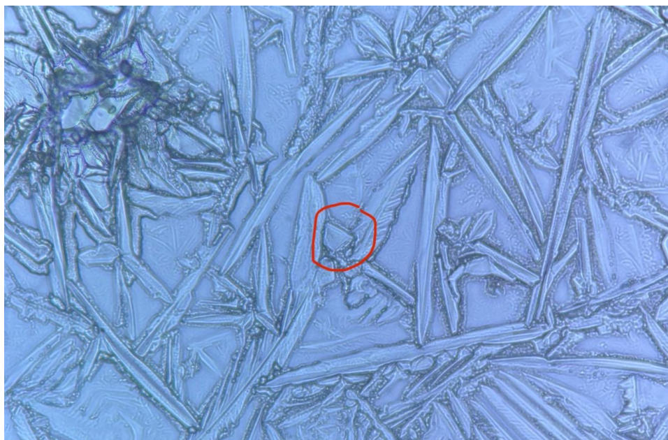
Figure 7. Optical microscopy of polystyrene standard diluted with KOH under 40x magnification.
